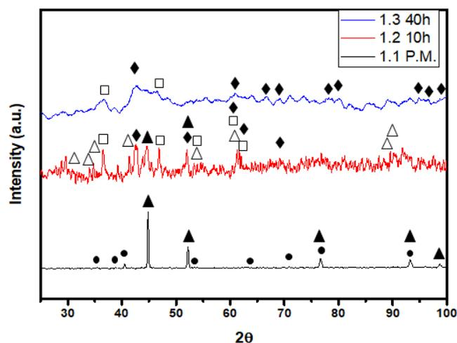
Fig. 1. X-ray diffraction pattern of samples 1.1, 1.2 and 1.3; ▲Ni, ●Ti, ◆NiTi, □TiO<sub>2</sub>, ▽Ni<sub>2</sub>Ti<sub>4</sub>O
