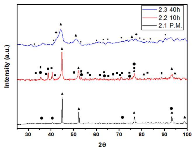
Fig. 2. X-ray diffraction pattern of samples 2.1, 2.2 and 2.3; ▲Ni, ●Ti, ◆NiTi, ■NiTiO<sub>3</sub>, ★NiTi<sub>2</sub>
