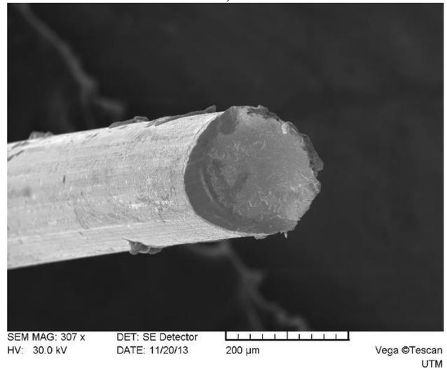
Fig. 4. SEM images of tool-electrodes made of W+Re10% that participated in the treating process:  $U=60V$ ,  $C=200\mu F$ ,  $\varnothing_{tool}=\varnothing_{piece}=0.2mm$ ;  $S=0.2mm$ ,  $n>1$ ; a) the tool-electrode connected as anode; b) the tool-electrode connected as cathode
