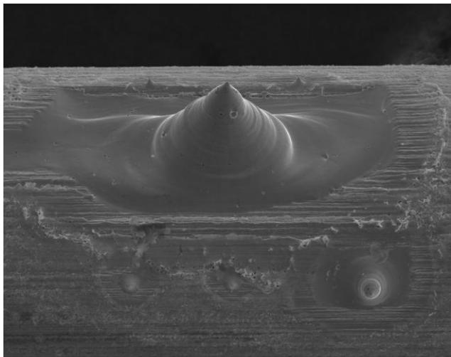
Fig. 3. Scanning electron microscope (SEM) image of a conic asperity surrounded by smaller ones, extracted on the surface of the piece material at a solitary discharge (the piece and the tool-electrode being made of W+Re10% as cylindrical wire with a diameter of 0.2mm, the condenser battery charged at the voltage  $U=70V$ ; the capacity of the condenser battery is  $C=200\mu F$ , the interstice having the value  $S=0.2mm$ )
