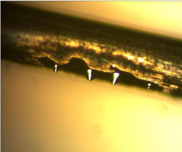
Fig. 5. Optical image of piece electrodes that participated in the treating process: W+Re 10%; U=60V; C=200 $\mu$ F; S=  $\varnothing_{\text{tool}}=\varnothing_{\text{piece}}=0.2\text{mm}$ ; n=2.
