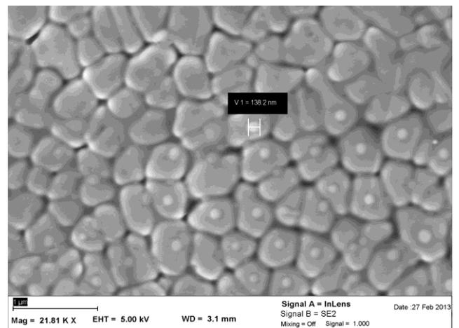
Fig. 9. SEM image of mosaic blocks on the lateral surface of a Taylor shape cone.
