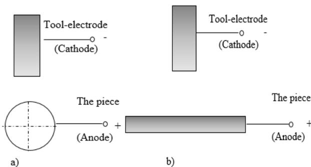
Fig. 2. Schemes of electrode positioning used in the experimental investigations and their connection in the circuit of power impulse generator discharge: a) the case of cylindrical piece; b) the case of flat piece.
