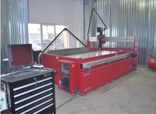
Fig. 8. The Maxiém Waterjets water jet-cutting machine, [12]
