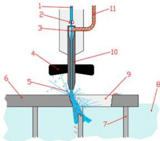
Fig. 4. Scheme of equipment for abrasive water jet cutting (injection): 1 - abrasive water jet; 2 - nozzle; 3 - mix room; 4 - shields; 5 - hydro abrasive jet; 6 - workpiece; 7 - lattice support for workpiece; 8 - water tank; 9 - piece cut; 10 - combination tube; 11 - abrasive particles
