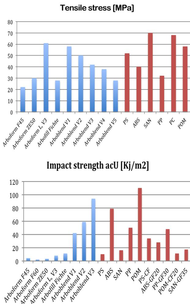
Fig. 1. "Liquid wood" vs. conventional plastic, [5]: ABS = Acrylonitrile butadiene styrene; SAN = Styrene-acrylonitrile resin; PP = Polypropylene; PC = Polycarbonate; POM = Polyoxymethylene
