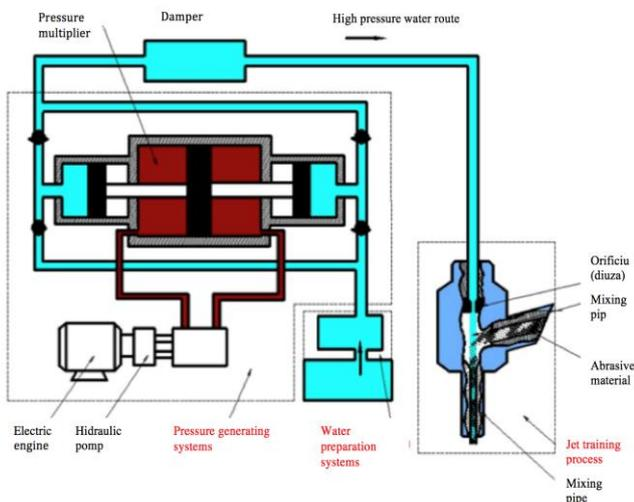
Fig. 6. The design of the abrasive water jet cutting machine, [10]
