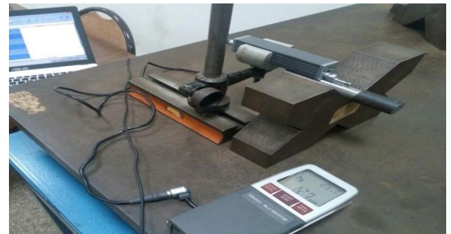
Fig. 2. Surface roughness measurement
