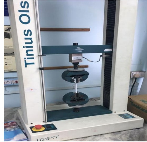
Fig. 2. 25kN Universal testing machine used for the mechanical tests
