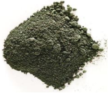
Fig. 3. As received SiC nanopowder
