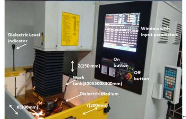
c) Electrical Discharge Machine Used for Experimentation Fig. 1. Electrode materials and the machine used for Electric spark machining process
