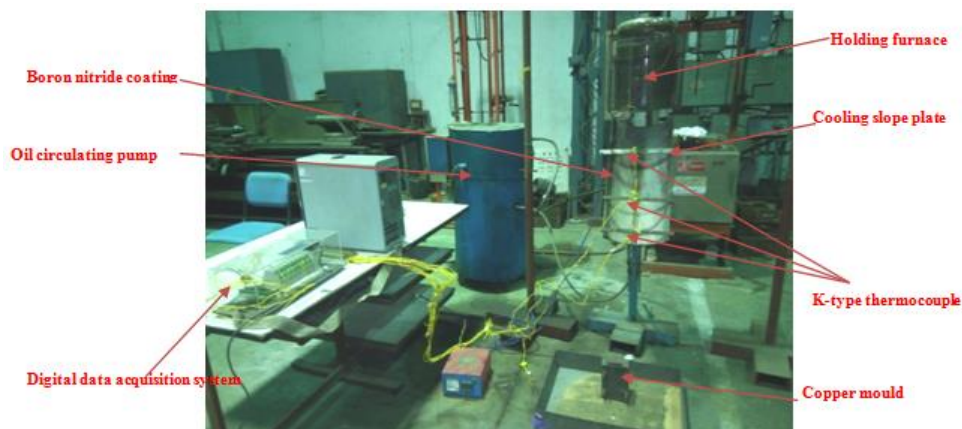
Fig. 2. Experimental setup of cooling slope techniques
