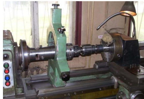
Fig. 5. Device for skiving hydraulic samples with MTB
