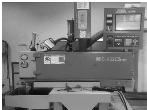
(a) Die-sinking EDM set-up
