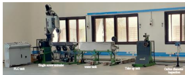
Fig. 2. A pictorial view of single screw extruder set up
