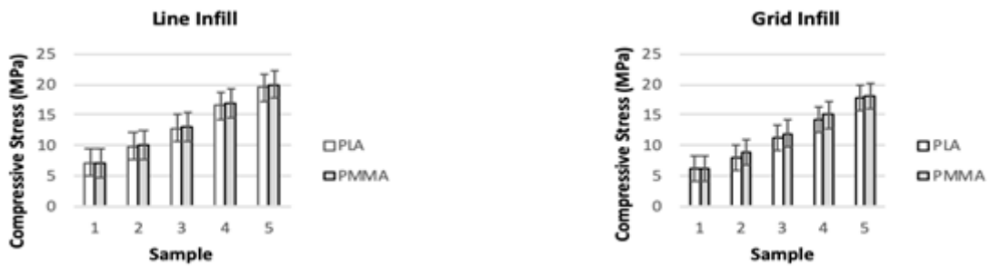
Fig. 11. Compressive strength for both experiments. (a) Compressive strength for grid infill (b) Compressive strength for line infill
