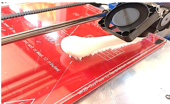
Fig. 15. Printing process using PMMA material with controlled porosities at ratio 1:0.7
