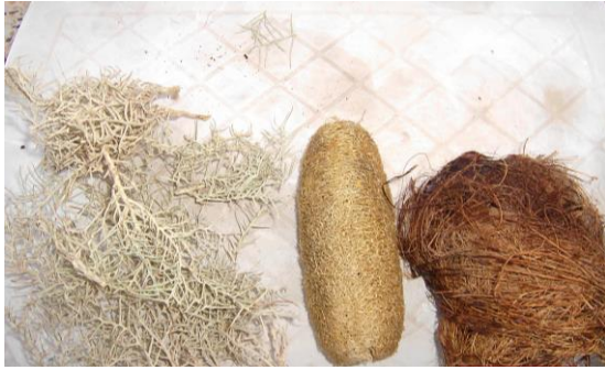
Fig.3. Sample of each of the filling medium to be tested in the trickling filter model; from left to right Wild Thorn, Arum and Date palm Bark
