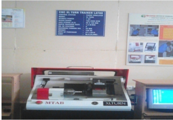
Fig. 1. Experimental set up using XLTURN- CNC lathe
