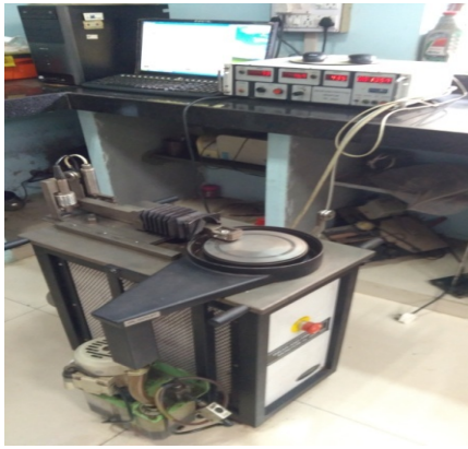
Fig. 5. Pin on disc experimental set up of for wear testing
