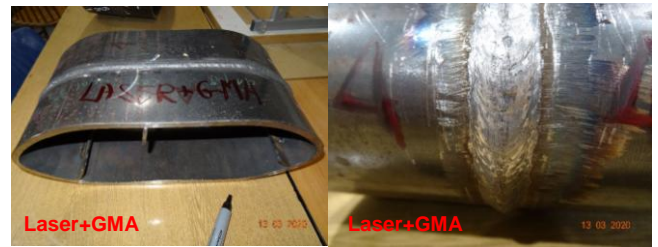
Fig. 14. A view of welded butt joints of API 5LX80, 323.9 mm diameter, 10 mm wall thickness tubes after flattening tests
