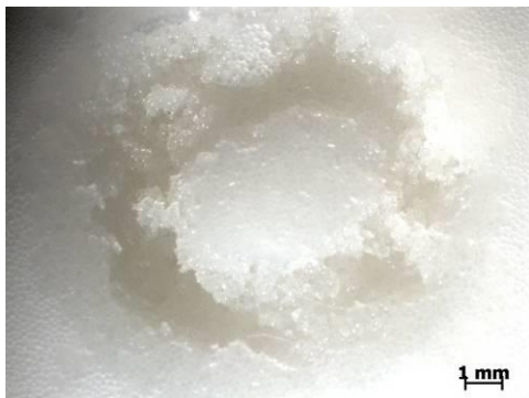
Fig. 14. Heavy degradation of the surface of the sample polymerized at 60°C, magnification 10x
