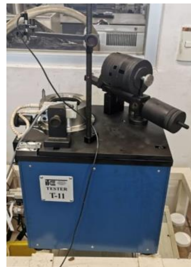
Fig. 6. T-11 Pin-on-disk tribotester
