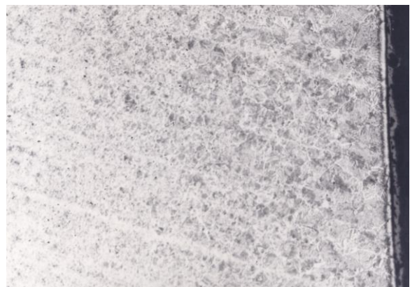
Fig. 3. Microstructure at the argon - nitrogen plasma cut surface
