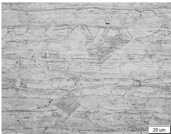
Fig. 6. Microstructure of AISI 304 stainless steel after 10% of deformation, Etching- Mi17Fe
