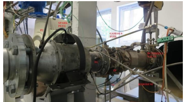
Fig. 2. Combustion chamber assembly and pressure regulation valve
