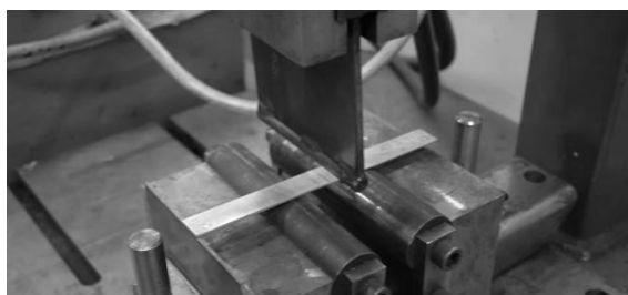
Fig. 3. A view of the device for technological bending test of 3.0 mm thick butt joints of AlSi1MgMn and its configuration
