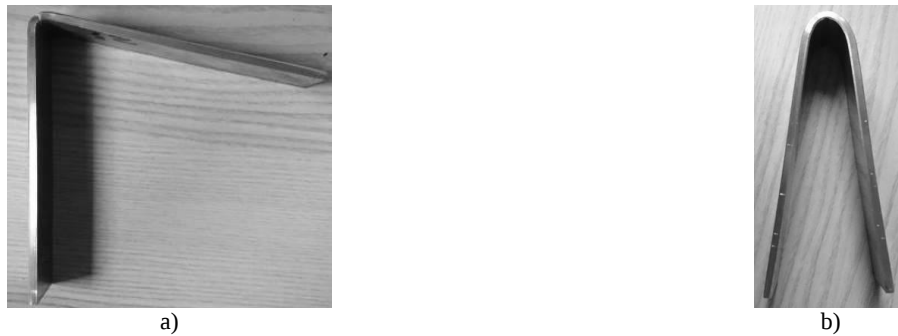
Fig. 4. A view of the samples of the butt test joint of AlSi1MgMn 3.0 mm thick sheets made at the energy input of 80 J/mm; a) after weld face bending (crack at approx. 100°), b) after root bending (full angle 180°)
