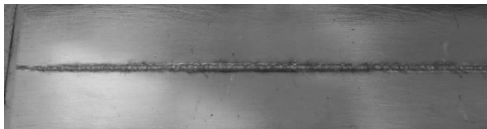
Fig. 2. A view of a representative test joints of AlSi1MgMn 3.0 mm thick and 200 mm long sheets made at the laser beam power of 2.0 kW and welding speed 1.5 m/min (energy input 80 J/mm)
