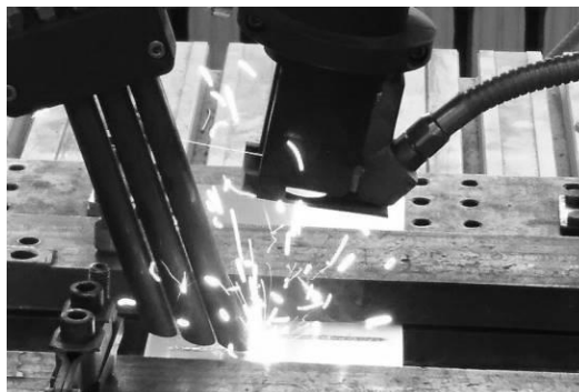
Fig. 1. A view of bead-on-plate laser welding of aluminium alloy AlSi1MgMn by the TruDisk 3302 laser (head tilted at 12°)
