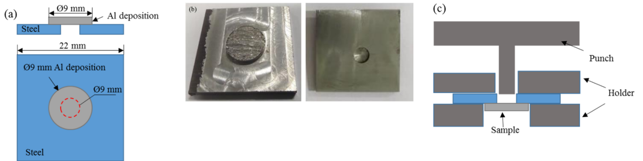
Fig. 3. (a) Schematic diagram (b) actual image of the push-off test specimen and (c) fixture arrangement on universal tensile testing set-up
