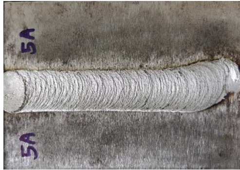
Fig. 2. Friction surfacing deposited sample
