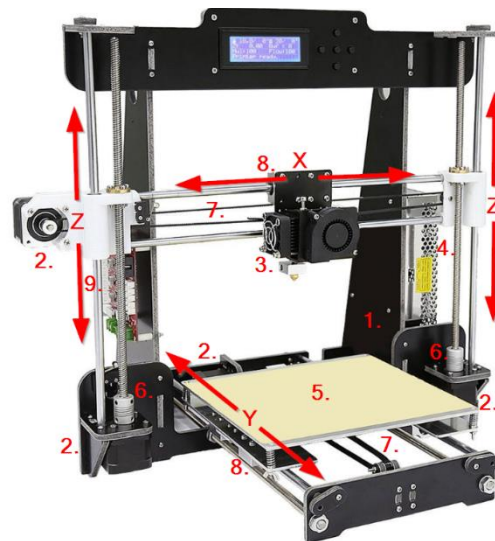
Fig. 1. 3D printer base structure built on an acrylic frame. 1- structure frame, 2- stepper motor, 3- extruder, 4- power supply, 5- platform, 6- coupling, 7- drive belt, 8- linear bearings, 9- motherboard.
