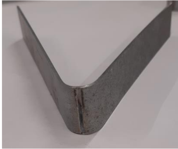
Fig. 7. A view of the joints after bending test
