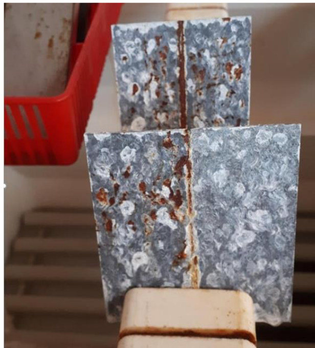
Fig. 11. View of the samples during the salt spray test after 96h
