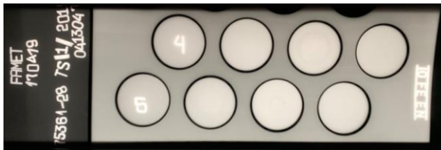
Fig. 8. A view of the test plate after RT examination of the fourth and fifth row of joints
