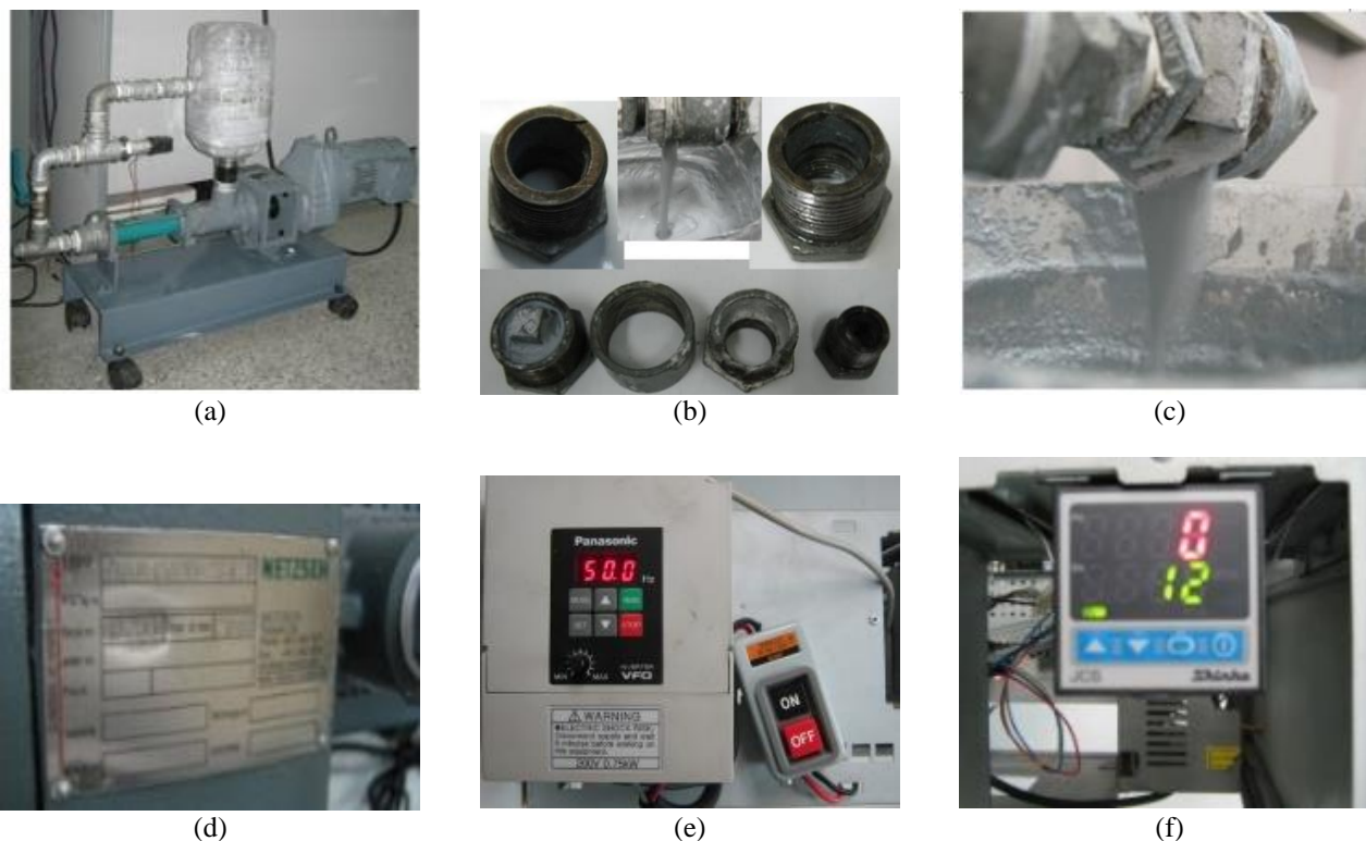
Fig. 2. Display (a) One-way AFM prototype, (b) workpiece holder (c) flow of abrasive media (d) nameplate of motor, (e) inverter control, (f) pressure display
