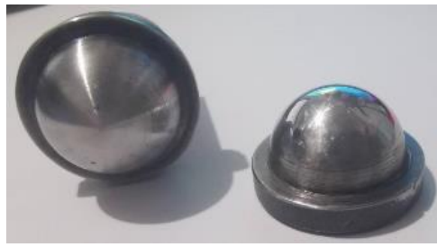
Fig. 3 SKD61 (AISI H13) Workpiece of AFM prototype
