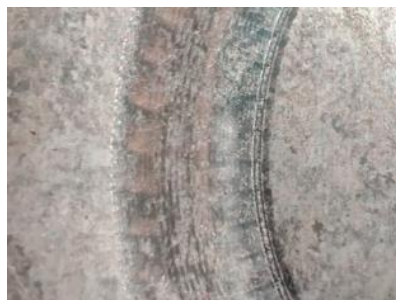
Fig. 8. Smooth macrostructure at the optimal solution avoiding the chipping
