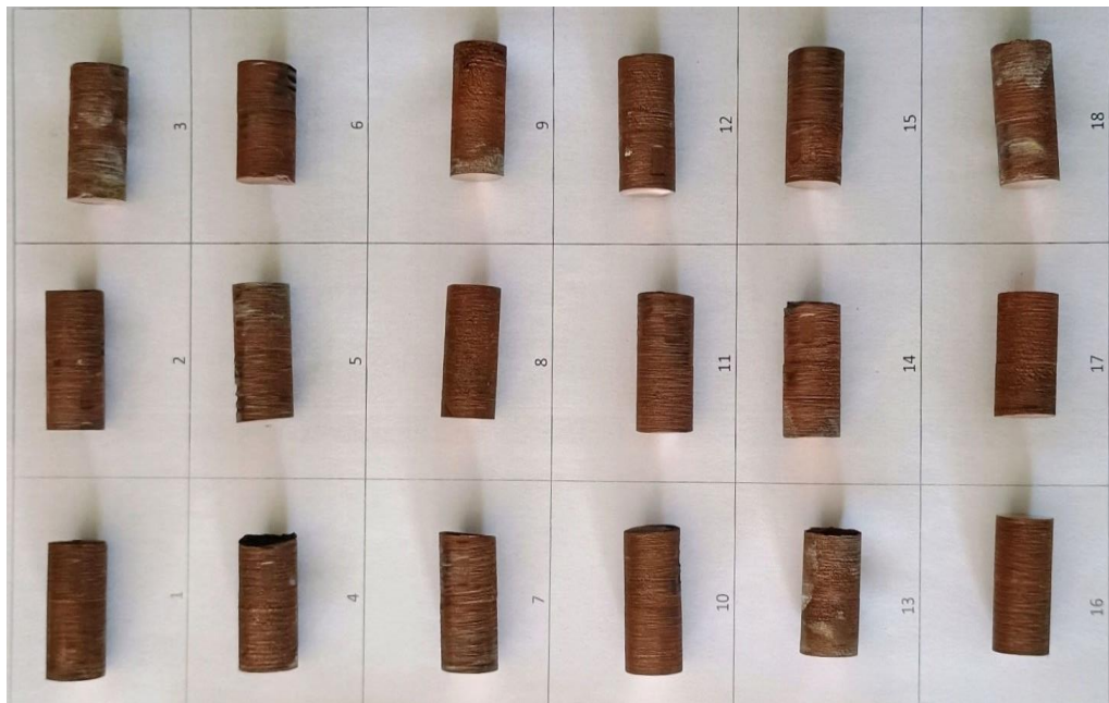
Fig. 2. Sintered copper pins after machining
