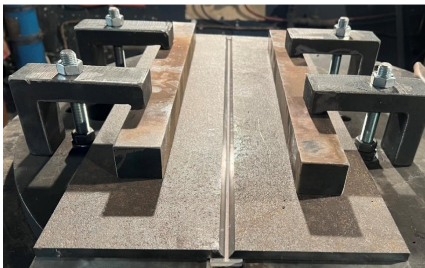
Fig. 1. A view of test plate with a ceramic washer mounted on the robot's welding table
