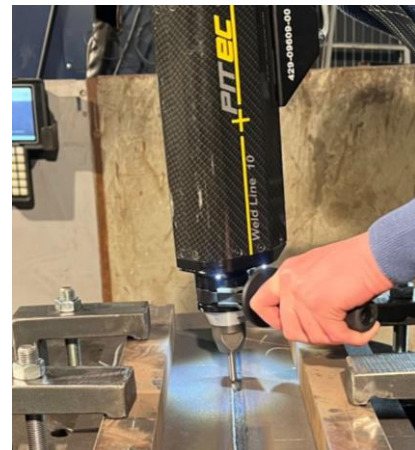
Fig. 5. Peening of a weld of a test plate process
