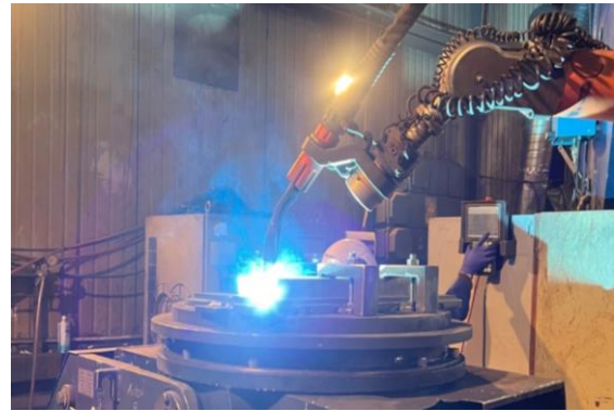
Fig. 3. A view of the welding process on the robotic station
