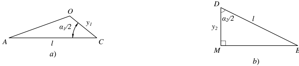
Fig. 14. Calculation of the offset of characteristic points on the support belt when the knife contacts the surface of the leather fabric of the skin (a) and when the rod and support belt contact from below (b)
