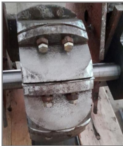
Fig. 17. General view of the proposed working drum of a staking machine for processing leather fabric of the fur skin
