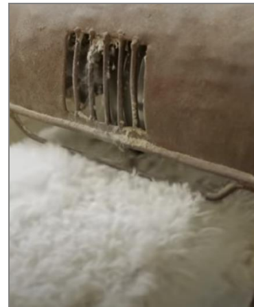
Fig. 18. The process of staking the sheepskin (grain face)
