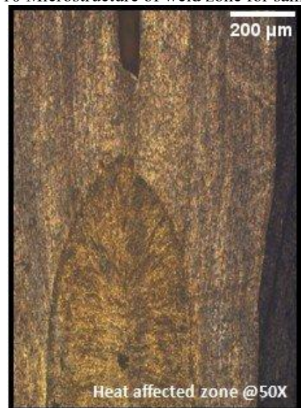
Fig. 12 Microstructure of weld zone for sample 5
