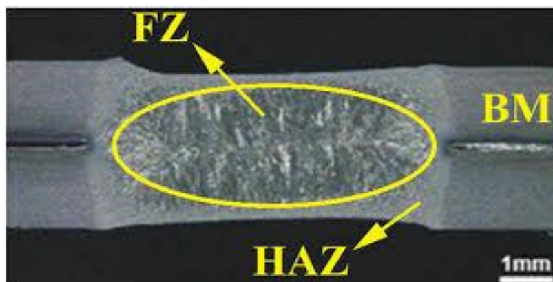
Fig. 6. Micrograph showing different regions in the RSW joint of 316L steel
