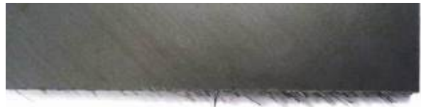
Fig. 2.7. Typical delamination of a milled unidirectional CFRP material
