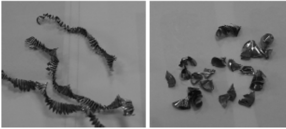
Fig. 4.10 Chips without chip breaker geometry (left) and chips with chip breaker geometry (right)
