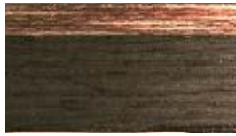
Fig. 2.3. Combination of Unidirectional and woven CFRP
