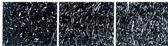
Fig. 27. Microscopic shots of hardwood fiber present in different quantities, [2]
