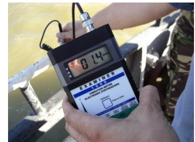
Fig. 5. Vibrations transmitted to the manrope - main deck
