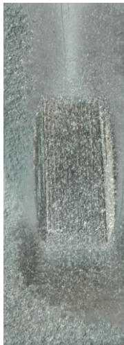
Fig. 8. View of the samples after the test surface abrasion
