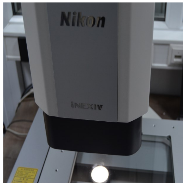
Fig. 9. The microscope Nikon® iNEXIV VMA-2520 type used for measurements
