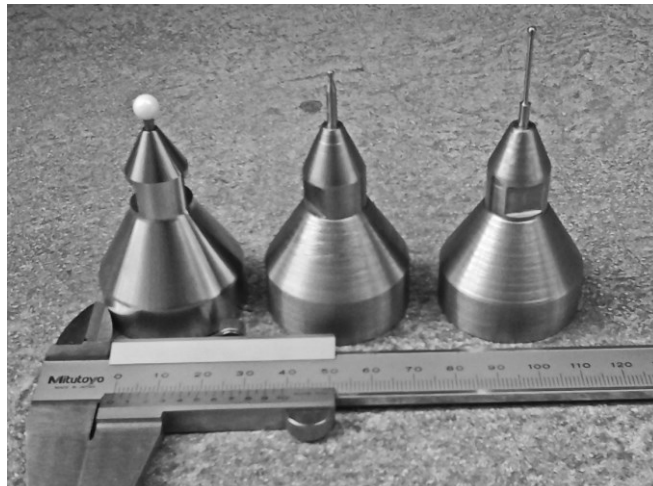
Fig. 3. Additional Faro® Edge cones for expanding measurement capabilities
