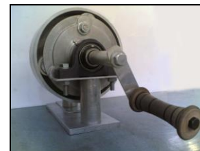
Fig. 1. The fabricated speed reducer after assembled
