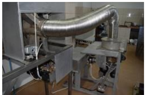
Fig. 3. Laboratory microwave experimental waste melting installation
