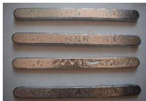
Fig. 4. Metal ingots recovered from white metals waste
