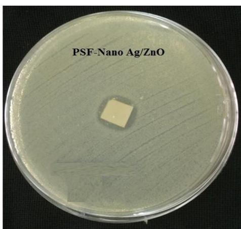
Fig. 7. Inhibition area of the bacteria used to examine the viability of the membranes as antibacterial
