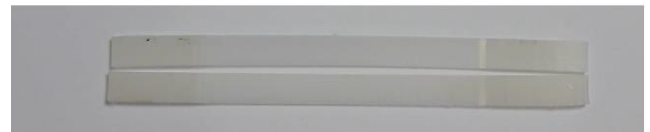
Fig. 2. Nylon tension specimens 3D printed according to ASTM D3039/D3039M – 14 [24]
