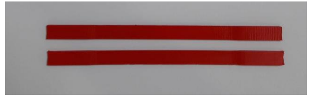
Fig. 1. PLA tension specimens, 3D printed according to ASTM D3039/D3039M – 14 [23]
