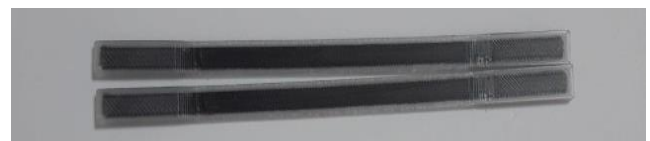
Fig. 3. Nylon-carbon tension specimens 3D printed according to ASTM D3039/D3039M – 14 [24]
