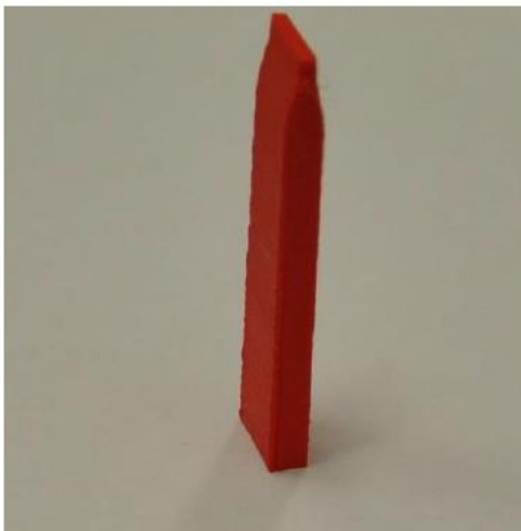
Fig. 6. Vertical building of the PLA sample on the printing bed
