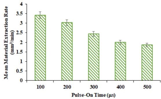
Fig. 6. Deviation in MER with pulse ON time
