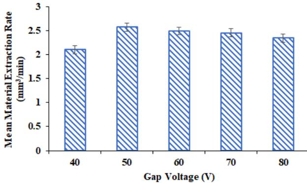
Fig. 5. Variation of MER with Gap Voltage
