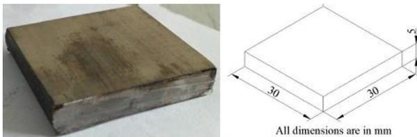
Fig. 1. AISI D3 steel workpiece
