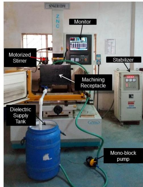
Fig. 3. PBESM Experiment Set up
