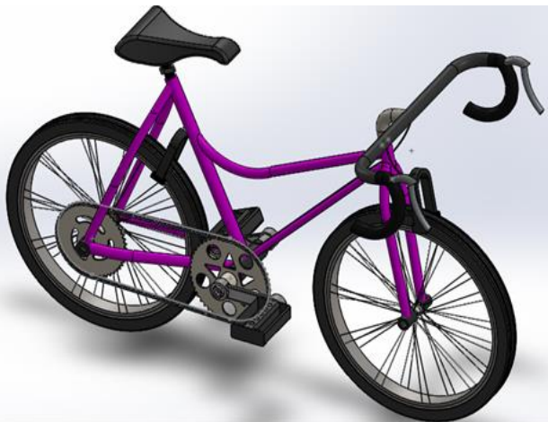
Fig. 8. The fully assembled model of a small frame bicycle
