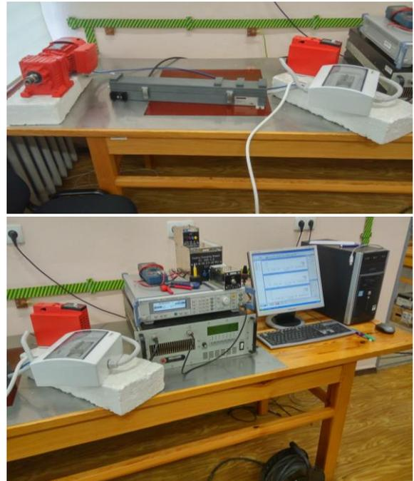
Fig. 2. Stand for testing the resistance for conducted disturbances with the use of EM (Electromagnetic Model) clamps together with the frequency converter and the electric motor
