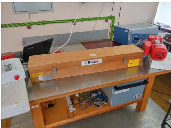
Fig. 1. Stand for testing the resistance for conducted disturbances with the use of CDN (Charge Device Model) clamps together with the frequency converter and the electric motor
