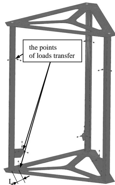
Fig. 9. The defined boundary conditions in relation to the frame element
