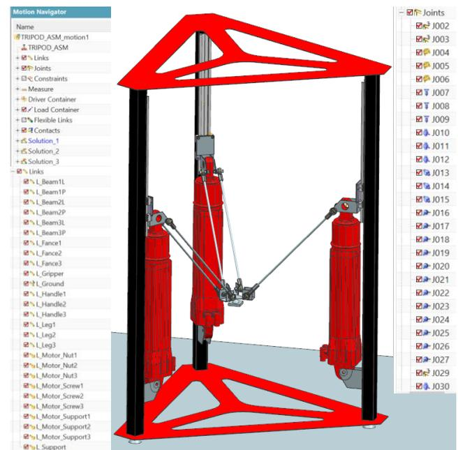
Fig. 4. The 3D model of the tripod system prepared for the motion simulation
