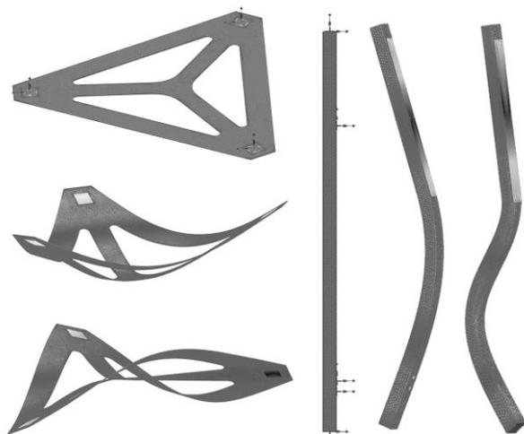
Fig. 15. The form of the frequencies of natural vibrations in relation to the pillar and platform of the frame
