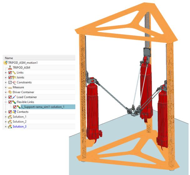
Fig. 8. The definition of flexible body type element
