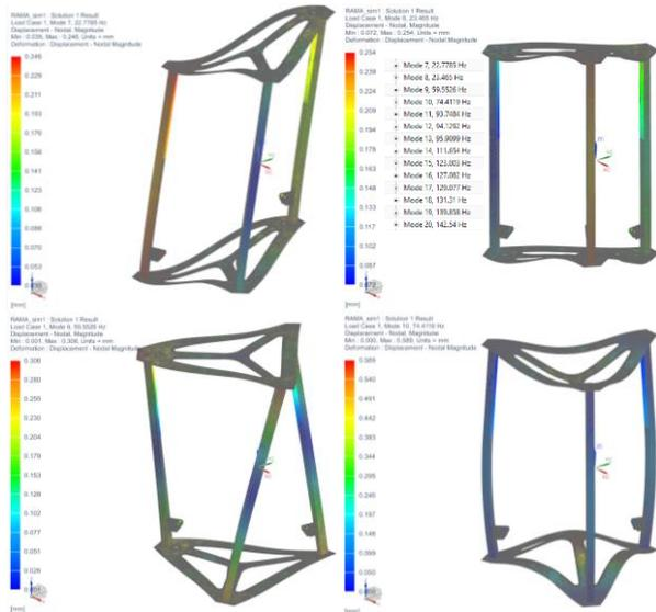
Fig. 10. Determining the frequencies of natural vibrations
