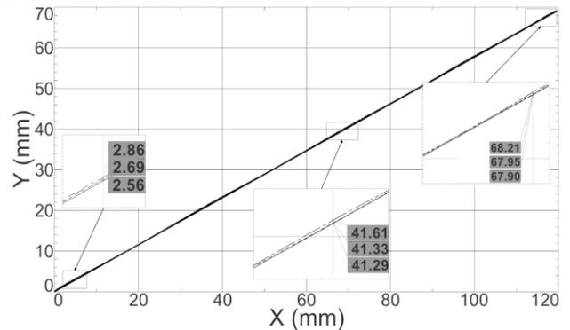
Fig. 13. The influence of the L dimension on the motion trajectory of the moveable platform
