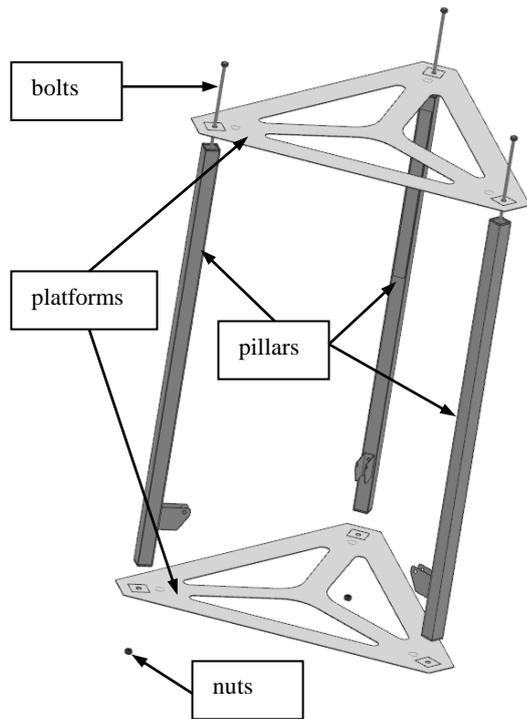
Fig. 14. The system model including bolted connection
