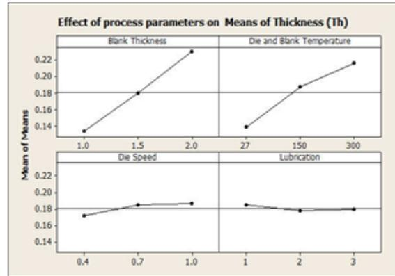
Fig 4. Effect of process parameters on Means of Thickness (Th)
