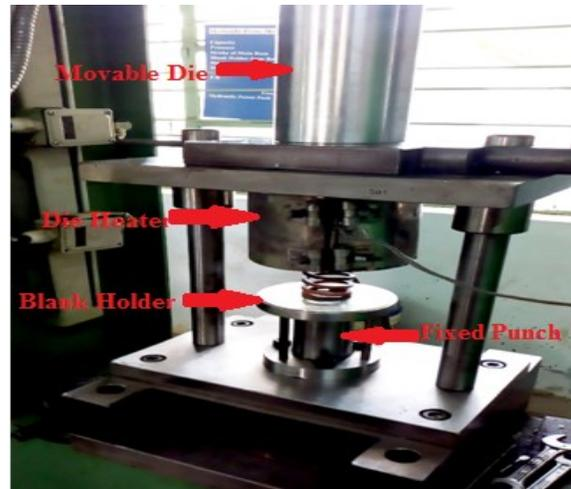
Fig. 1. Experimental setup for forming tests
