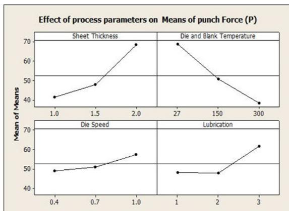
Fig 3. Effect of process parameters on Means of Punch force (P)
