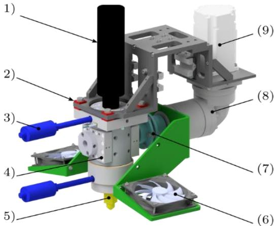
Fig. 4. Print head: (1) Heated flexible tube, (2) Thermal insulation, (3) Pressure sensor, (4) Gear pump, (5) Nozzle, (6) Fans, (7) Clutch, (8) Gearbox (9) Servo motor
