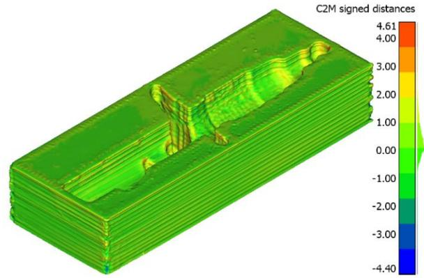
Fig. 7. Cargo carrier shape deviation
