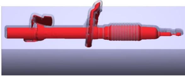
Fig. 5. Shock absorber with transparent offset surface and the resulting cargo carrier
