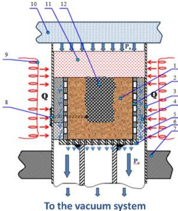
1- a mould; 2- a perforated flask; 3- a steel shell; 4- a thermo-insulation seal; 5- a fireproof insert; 6- a fireproof stand; 7- a fireproof plate; 8- a thermocouples; 9- a heaters; 10- a fireproof insert; 11- melt; 12- melt (matrix) and reinforcement phase particles.
