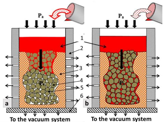
Fig. 1. Infiltration of the melt (the matrix) in the capillary spaces between the elements of the reinforcement phase: a- at the beginning of the pouring; b- after completed infiltration
