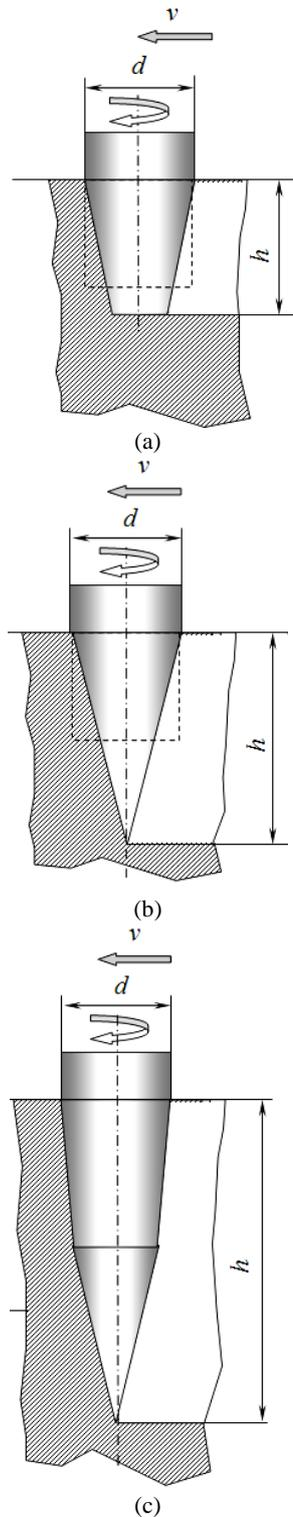
Fig. 5. The nature of the recess being formed and the change in the shape of the electrode depending on the speed of movement of the tool electrode:
