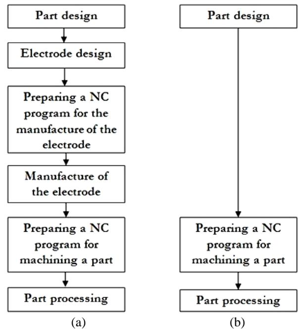
Fig. 6. The structure of the preparation cycle for EDM of a part during volumetric duplication (a) and during EDM with a rotating non-profiled electrode-tool (b)
