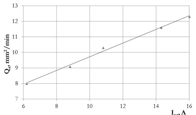
Fig. 4. Effect of short-circuit current ( $I_{sc}$ ) on cutting performance ( $Q_s$ )
