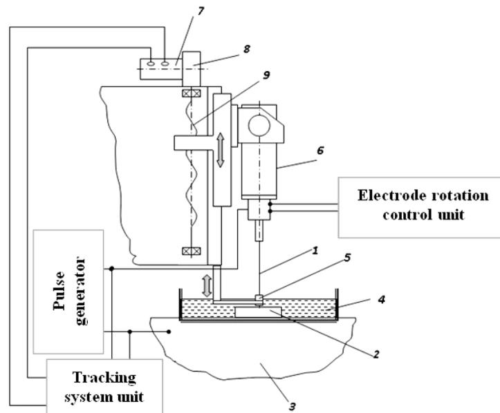
Fig. 2. Diagram of a module for electrical discharge machining with a rotating non-profiled electrode tool: 1 – wire electrode tool; 2 – processed product; 3 – table; 4 – bath; 5 – conductor sleeve; 6 – head; 7 – electric motor of the tracking system; 8 – reducer; 9 – lead screw
