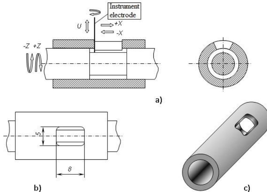
Fig. 3. Cutting out a hole in a tubular part: (a) processing scheme; (b) sketch of the treated surface; (c) tubular part with cut out hole
