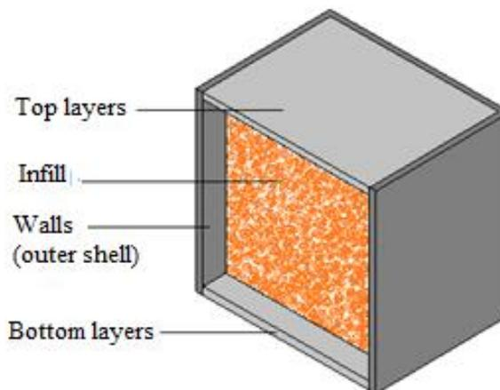
Fig. 3. Filling density inside the outer shell
