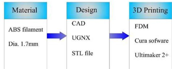
Fig. 6. Preparing 3D printing specimen
