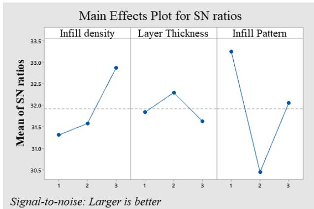
Fig. 11. S/N ratio for tensile strength
