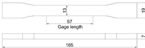
Fig. 5. Printed dog-bone shaped specimen
