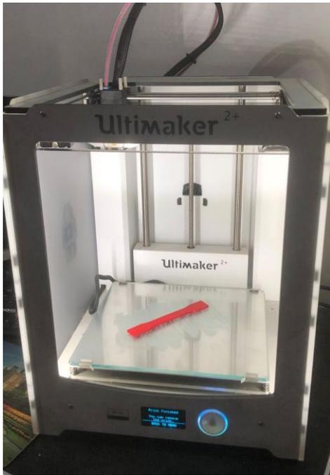
Fig. 8. Ultimaker 2+ FDM Machine
