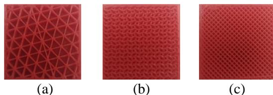
Fig. 2. Infill: (a) triangle, (b) gyroid, (c) line
