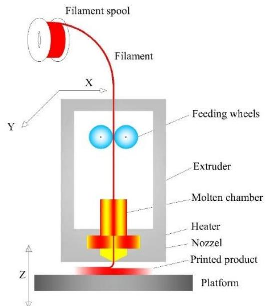
Fig. 1. Schematic diagram of the FDM printer
