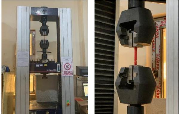
Fig. 9. Tension Testing Machine
